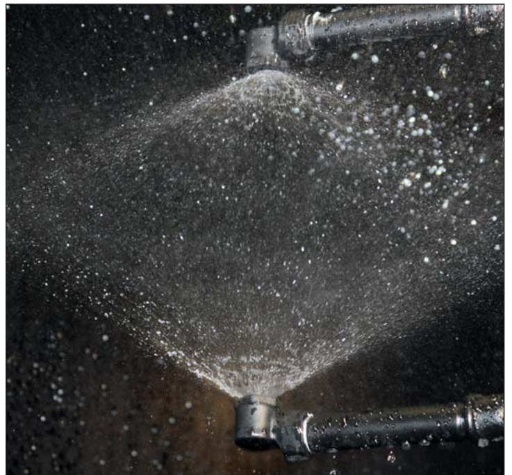
Special arrangement of nozzles for a high separation of dust and NH 3
